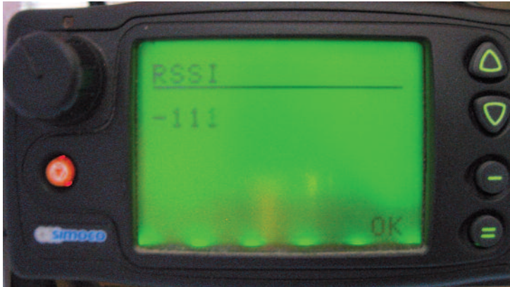
PHOTO 1: A poor noise floor of -111dBm at 70.450MHz, as indicated on a Simoco MA-9030 PMR radio.
